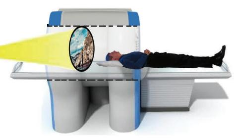
Screen attached to the cradle with short fixed distance to the subject to create wider field of View (FOV).
